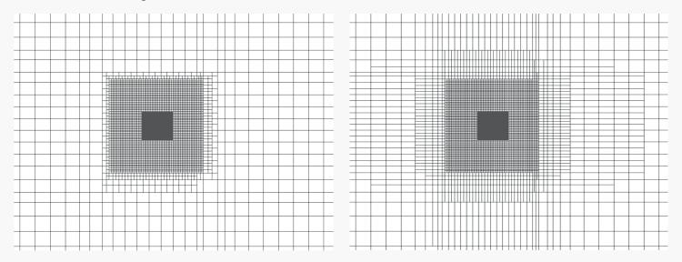
Above left: Refinement Slowdown is set to 1. No additional cells are added, and so there is no lengthening of the transition from fine to coarse grid cells.
