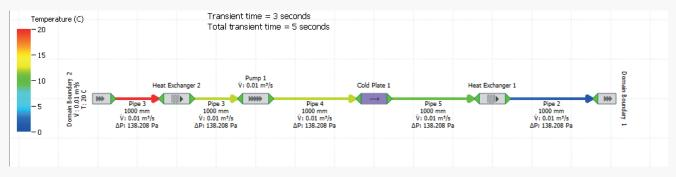
You have the option to model either air or liquid side flow networks. The flow network in the image above is a liquid side network, with the 1D cold plate object colored purple to indicate that it is connected to a cold plate in a 3D model. Standalone flow networks can be quickly solved using the dedicated Flow Network solver, while flow networks that are connected to a 3D model will be solved using the main solver.
