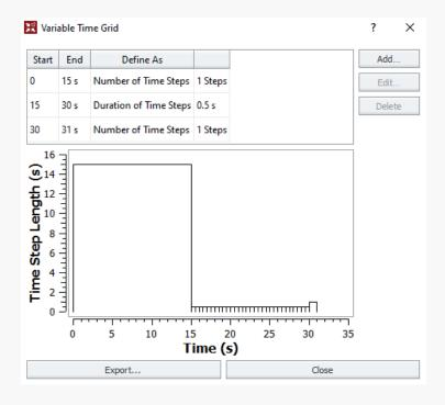
The Variable Time Grid Window (shown left) combines the time distribution graph and variable time grid.
